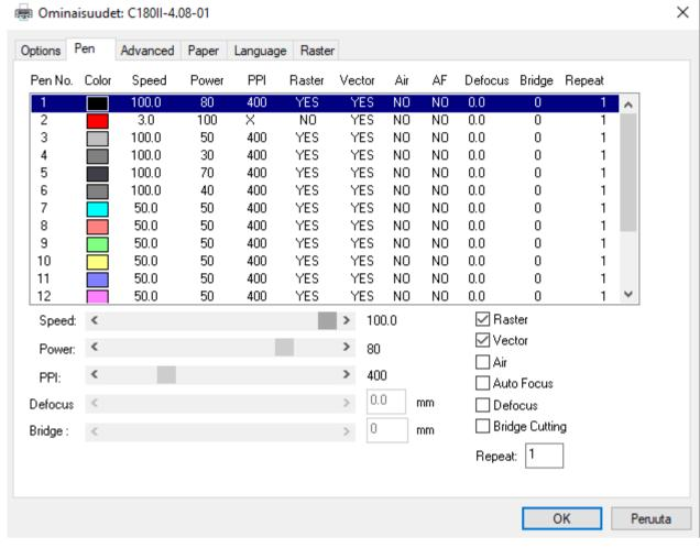
Speed-the controller sets the maximum allowed speed of the engraver's movement. The speed is also affected by, for example, the complexity of the engraved pattern. The laser cutter reaches 100% speed when cutting mostly straight lines.
