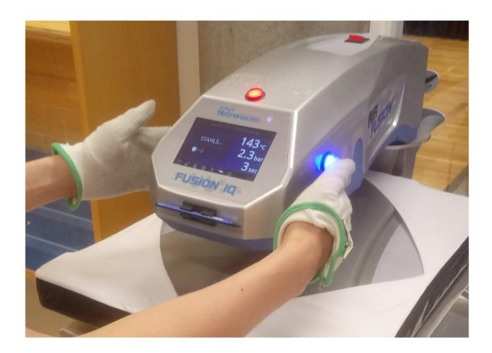
Pressing takes 5 seconds, after which the upper part automatically moves to the side.
