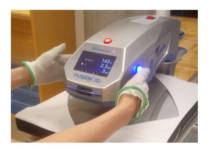
Pre-pressing takes 3 seconds, after which the upper part automatically moves to the side.
