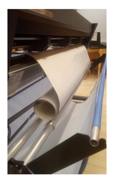
Place the sticker or vinyl so that the rollers holding the material in place are at the gray rectangles and as far as possible on the edges. Make sure the material is straight.
