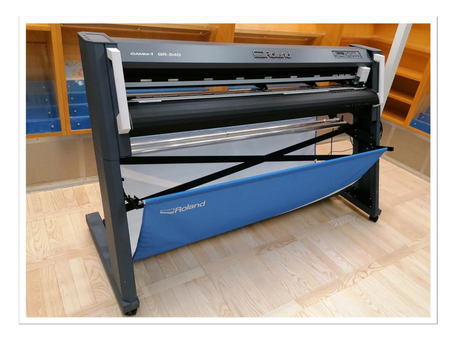
With the vinyl cutter you can create unique monochrome stickers and fabric prints. The sticker material is suitable for flat surfaces, such as windows, a bicycle or as a laptop decoration. The vinyl material is printed using a heat press to the canvas or fabric.
