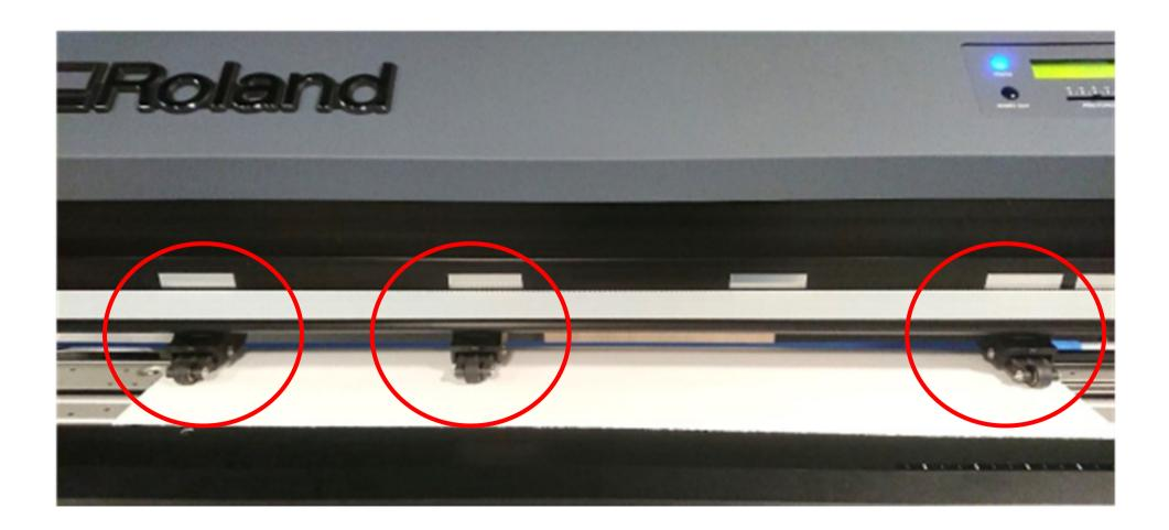
When the material is right, press the PINCH button on the device. The rollers descend and the material locks into place.
