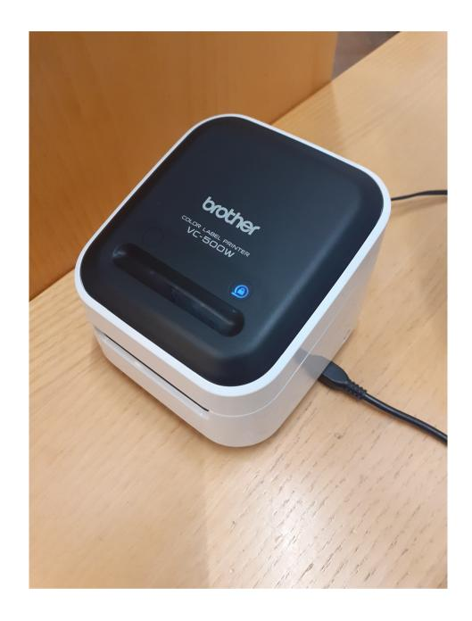
The sticker printer uses ZINK® Zero-Ink® printing technology, which means that no separate ink is needed. The color of the stickers is created by heat-activated color crystals, which the material contains.
