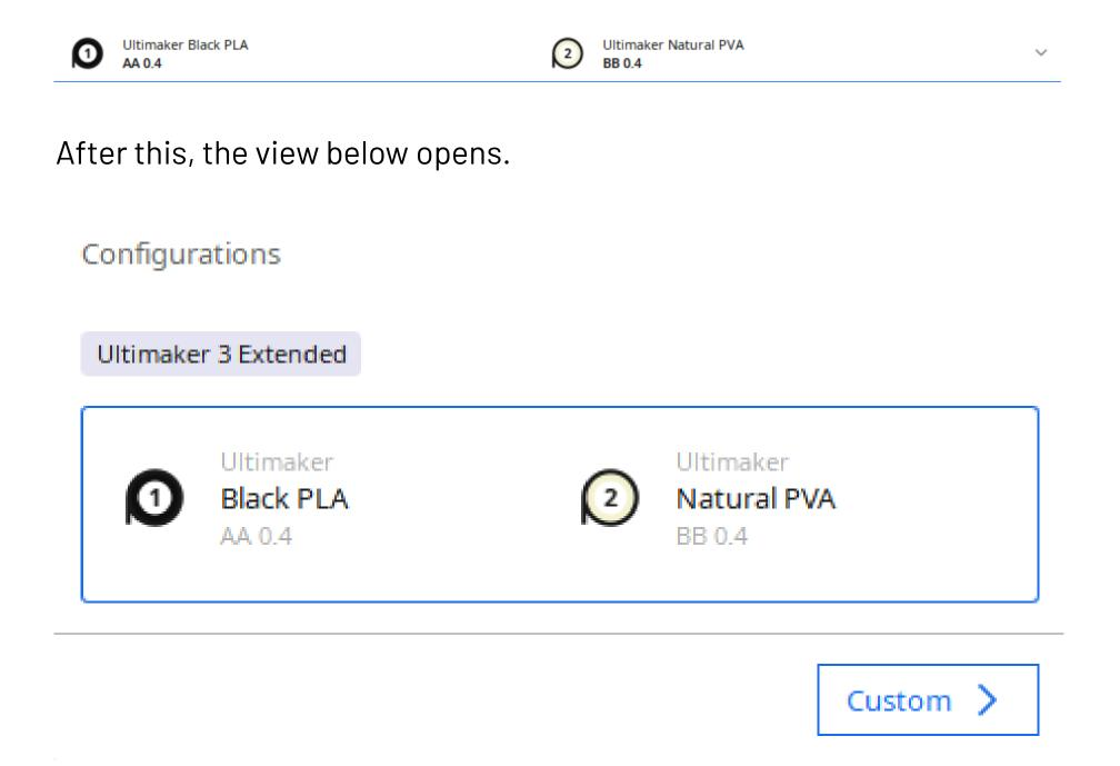
This shows the printer's current media settings. The materials must match, i.e. the material on the device must be the same color as the material shown in the Cura program. If the materials do not match, a message about an incorrect setting appears on the printer screen during the printing phase.
