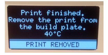
Wait until the print cores and the print bed have cooled down to at least 40 degrees. If there is too much heat, the print may warp or break. Remove the printout and clean up the resulting debris.
